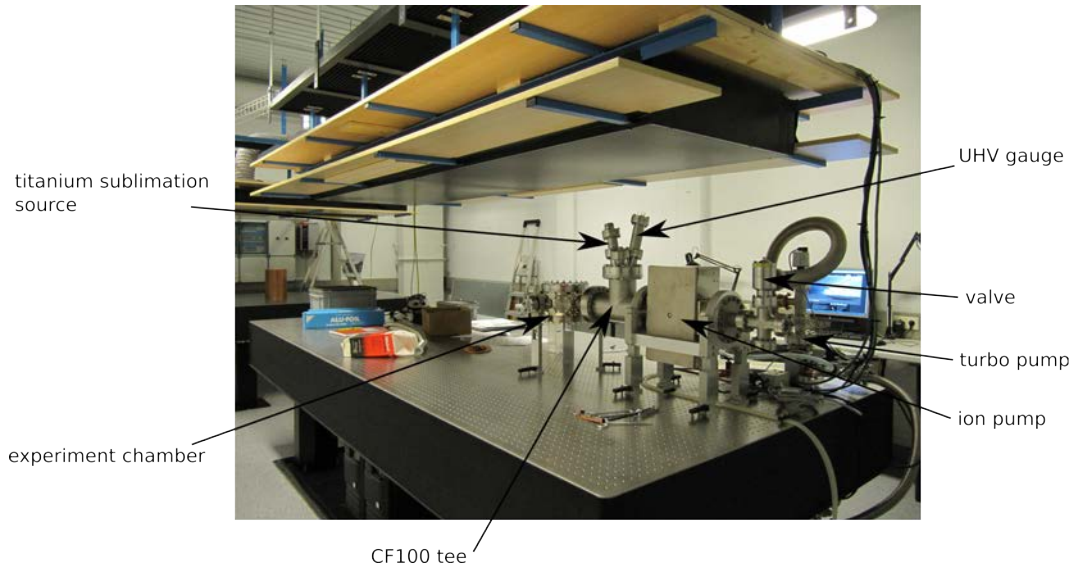
Figure 4.2: Vacuum setup prior to inserting the ion trap.
