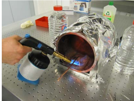
Figure 3.14: Picture taken during soldering. A piece of copper wire is soldered to the shield using an blowtorch.
